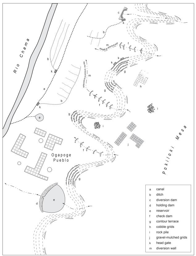
Figure 12-1. Idealized distribution of water and soil control features.
