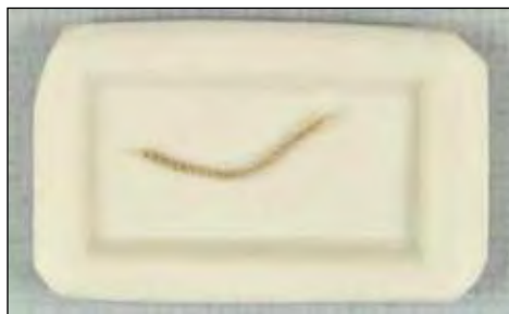
The same warp thread is shown after four plasma oxidations runs.
