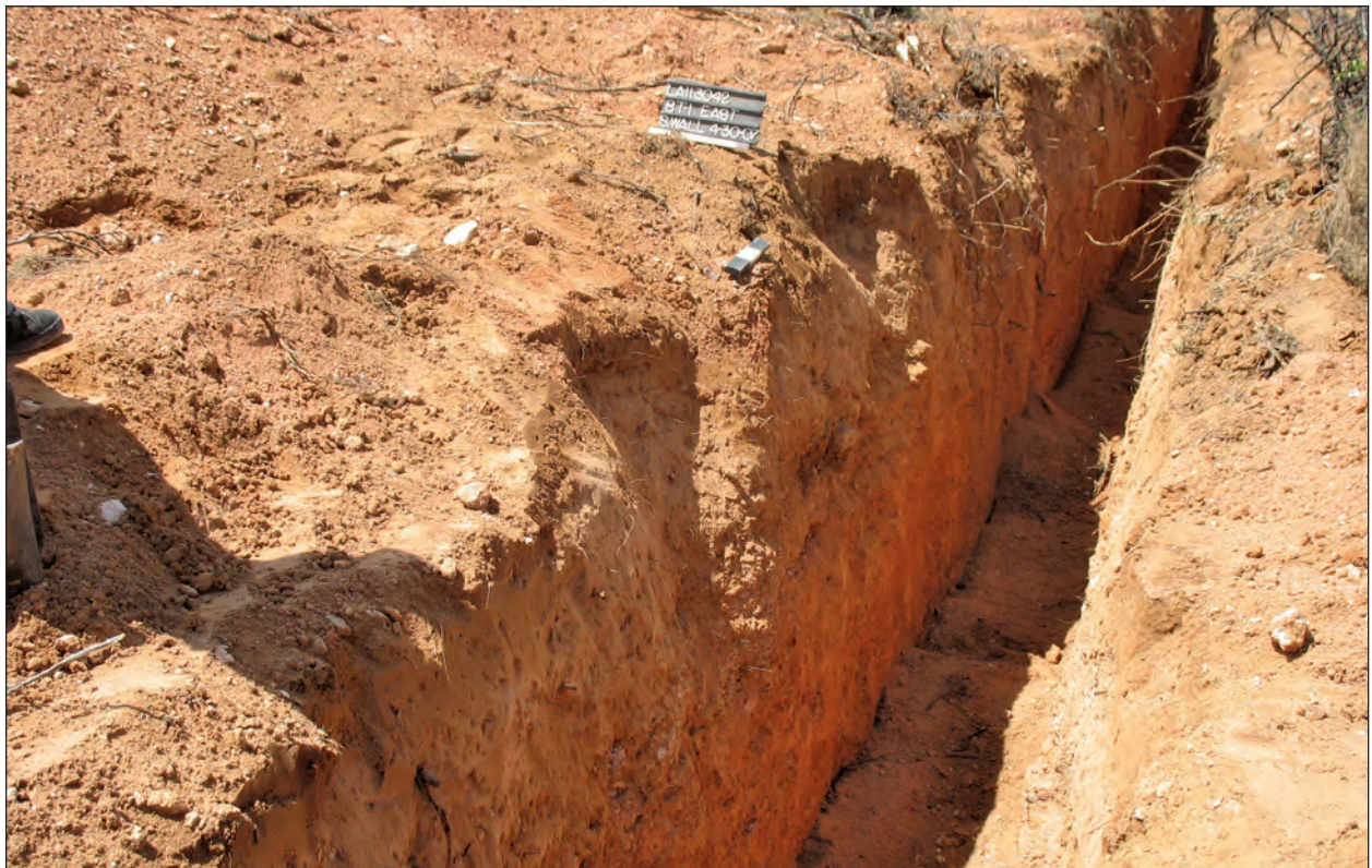
Figure 7.3g. LA 113042, BHT 1, south wall, profile. Recently redeposited eolian sand occupies the upper 3 to 5 cm, underlain by Bk horizon loamy sand.
