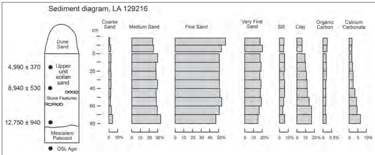
Figure 24.9. LA 129216, BHT 1, sediment data. The increase in amounts of clay and carbonate with greater depth is related to soil development.
