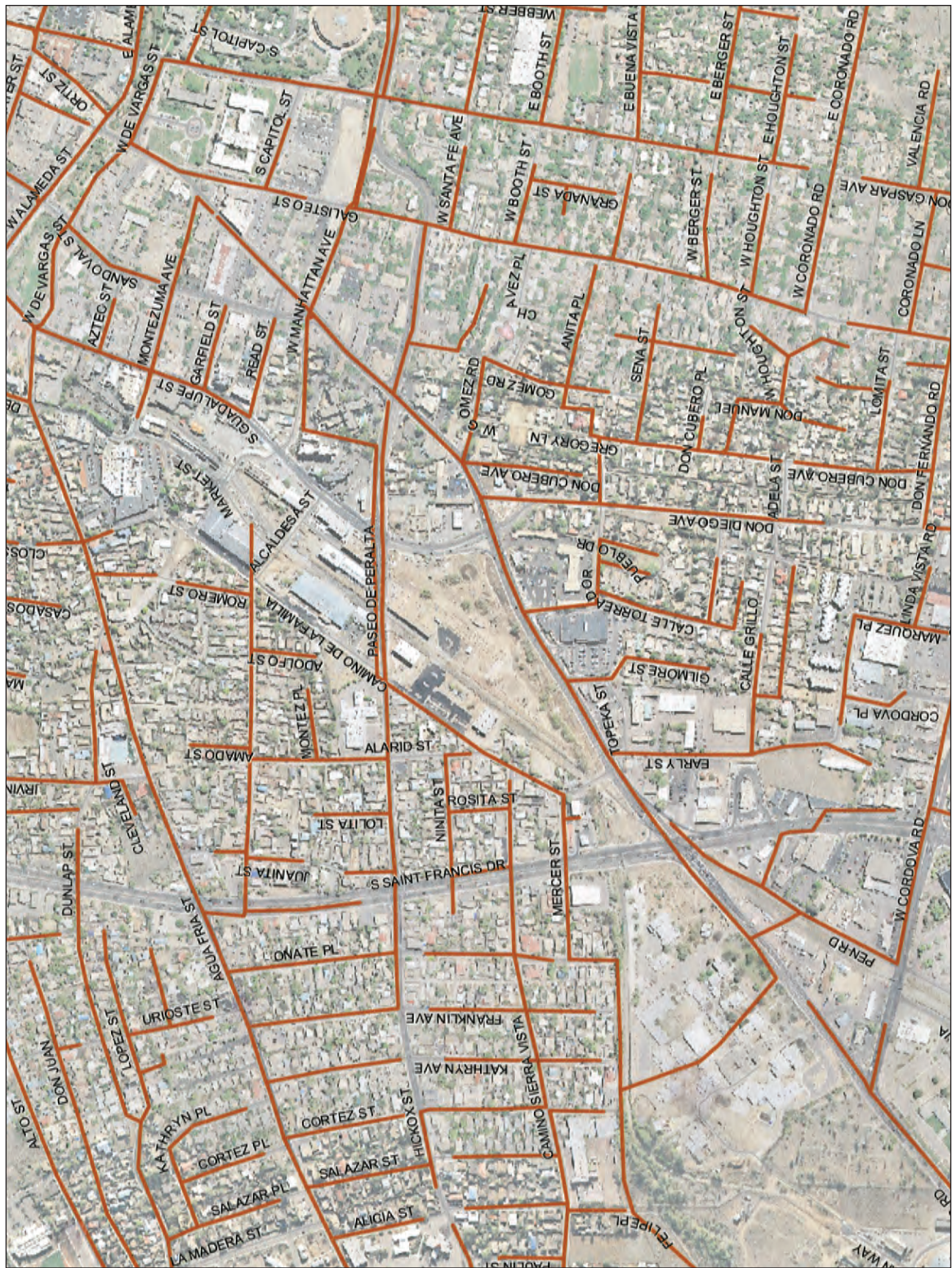
Figure 7.12. GIS map of Santa Fe's sewer systems, ca. 1990 (courtesy David Barsanti, Santa Fe, GIS Specialist, City of Santa Fe). Note that, although there are currently disjuncts across the railyards, several sewer lines appear to occupy former ditch laterals.
