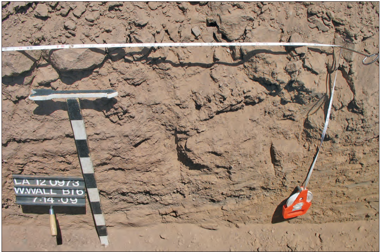
Figure 2.3. Soil profile of LA 120973, BHT 6. The upper, intact stratigraphic profiles revealed in some backhoe trenches and hand-excavated units consisted predominantly of massive silt with very fine to fine grained sand and variable clay development.
