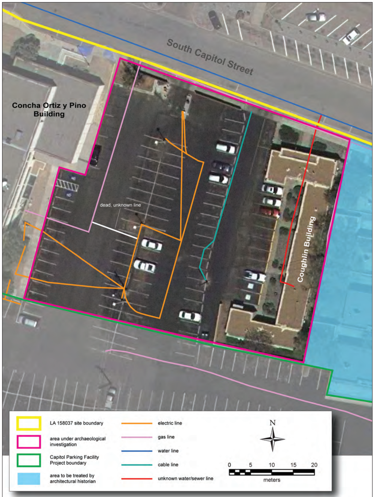
Figure 7.1. Plan view depicting the type and location of all known utilities within the project area.
