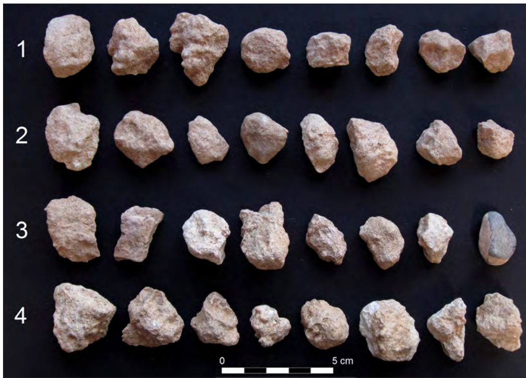
Figure 21.36. Small pebbles selected from the four gravel zones in the Jornada alluvium; all of these pebbles are dense caliche except the far right-hand pebble from zone #3, which is gray limestone (data in Table 21.15)
