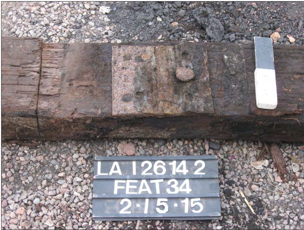
Figure 6.89. Railroad tie with metal tie plate and railroad spike removed from Feature 34.
